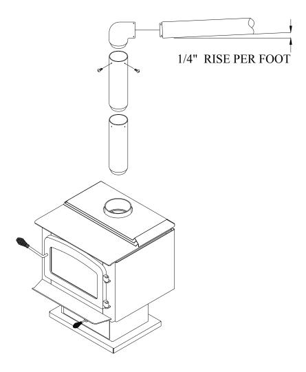
FIGURE 2.3 (B) Minimum Slope
